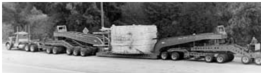
In 1979, a doughnut-shaped 107-ton superconducting electromagnet for SLAC arrives from Chicago on 120 wheels.
